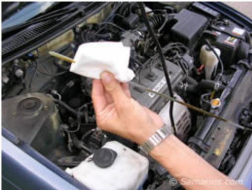
Wipe the dipstick off. Insert it back fully. Pull it out again and check the oil level.
