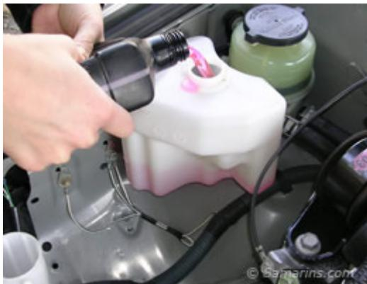
Add coolant only when the engine is cool. Use only recommended engine coolant. Sometimes engine coolant is sold already premixed with water and sometimes you will have to mix it. Check your owner's manual or read the directions on the coolant bottle. Carefully add the coolant into the overflow tank to make it between "LOW" and "FULL" marks.
