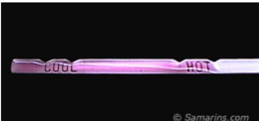
On most cars the new transmission fluid comes red (photo on the left). Over the time it becomes brownish, as in the photo below.
