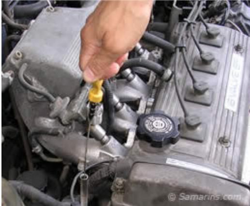
Park your vehicle on a level ground. Set the parking brake. Make sure the transmission is in "Park." Stop the engine. Wait for a minute or two to let engine oil drain into the oil pan. Pull the engine oil dipstick. If you don't know where it is located, check your [owner's manual](#), usually it has a bright handle saying "Engine Oil".
