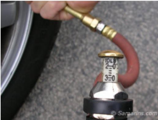
Pump or deflate to the recommended pressure. The maximum pressure listed on tires is NOT the proper pressure!
