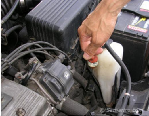
After the vehicle was driven for a while to let the transmission fluid warm up, place your vehicle on a level ground. Set the parking brake. Make sure the transmission is in "P" (Park) position. Leave the engine running. Find the automatic transmission dipstick (your owner's manual will tell you where it is located). Pull the dipstick out.
