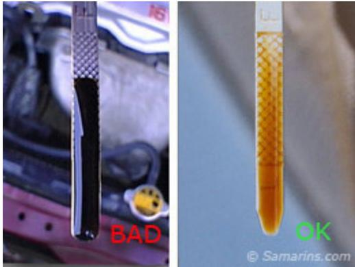
Check the oil condition: If it's way too black, as in the left photo, it's definitely time to change it. If it's brown, but still clean and transparent, as in the right photo, it's OK. If engine oil is of the "coffee with milk" color it means that engine coolant mixes with oil. This is a sign of some internal engine problem, such as, for example, a leaking [head gasket](#) - have your car checked out.
