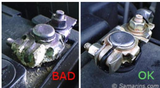
Check the battery condition visually. If you see any leaks, cracks or other damage, the battery needs to be replaced. Make sure the battery terminals are tight and not corroded.
