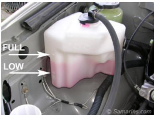
If the coolant level drops within a short time after topping up, there may be a leak. Have the
