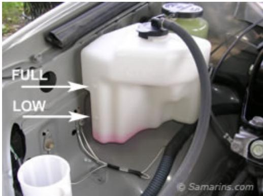
Visually check the engine coolant level in the overflow tank. Your owner's manual has the directions. The level should be between "Low" and "Full" marks. **(Don't open the radiator cap or the pressurized overflow tank cap when the engine is hot! The cooling system is under pressure when hot!)** If the coolant level is low, you can top it up using recommended type of coolant mixed with water. Again, your owner's manual has the proper way to do it.
