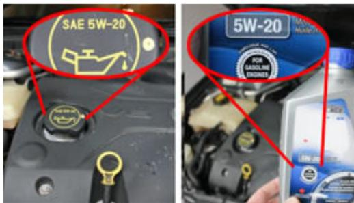
To top up engine oil use a recommended type of oil; for example, if your owner's manual or the oil filler cap indicates SAE 5W-20, use SAE 5W-20 oil. If your engine needs synthetic oil, use only synthetic oil. You can find the recommended oil type for your car in your owner's manual.
