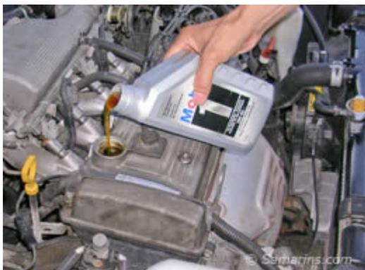
How to top up engine oil: Add a little amount of oil into the oil filler neck. Wait for a minute to let oil to flow into the oil pan. Check the oil level again with the dipstick. If it's still low, add some more. But don't overfill it. Don't forget to install the dipstick back and close the oil filler cap when you finished.
